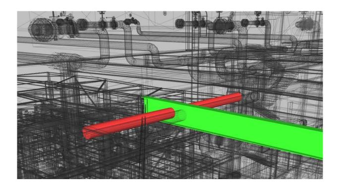
BIM coordination; Creation of a BIM model from 2D drawings; Collision checking
